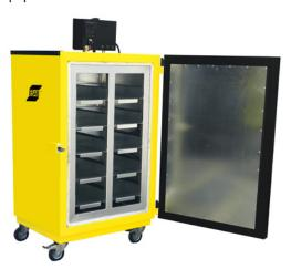
The SDE range of drying and storing ovens are large, thermally controlled cabinets designed specifically for welding electrodes. Ideally, a facility should have separate ovens for drying and storing. However with the SDE manual digital thermostat the same oven can be used for both drying and storing. Designed for stationary applications these come with heavy lockable castors to move around then lock in place. Aditionally a gas vent safely removes humidity and gases during the heating process.
